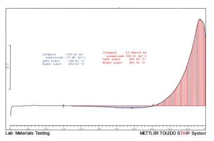
Figure 1. DSC Plot of Coffeen Fly Ash Sample
