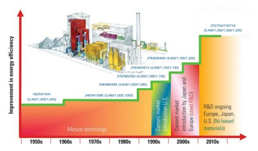
Above describes the Mainstream Pressure/ Main Steam Temperature/ Reheat Steam Temperature / Double Reheat Steam Temperature
