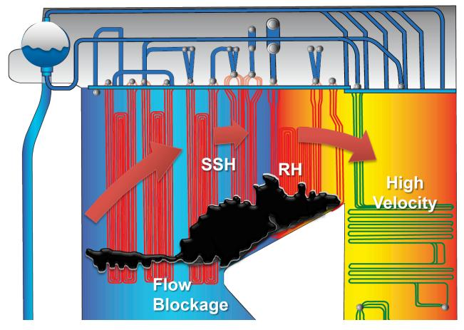
Non-Optimal furnace cleaning can significantly elevate the furnace exit gas temperature and forces heat to the convection pass .
