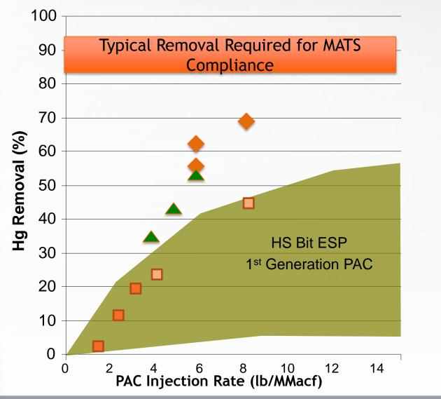
High Sulfur (2.8 wt%) Bituminous Coal Cold Side ESP
