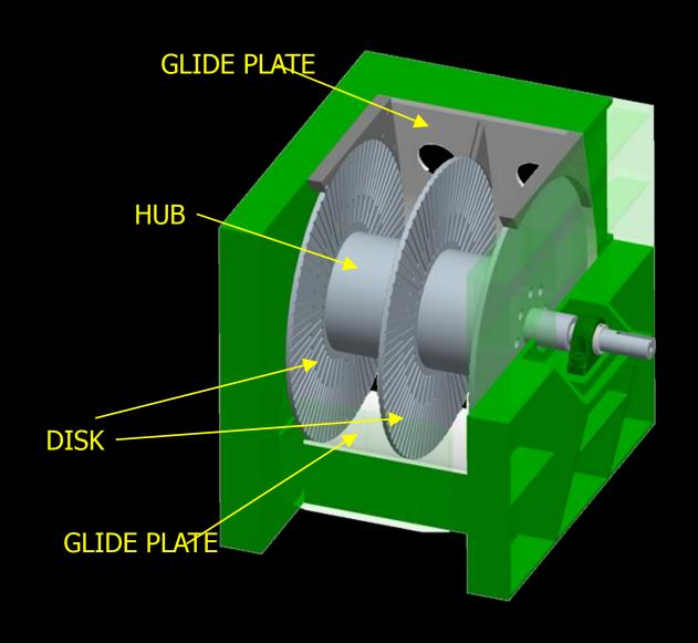
Feed material consolidates and locks up at a constant density as it enters the rotating duct
