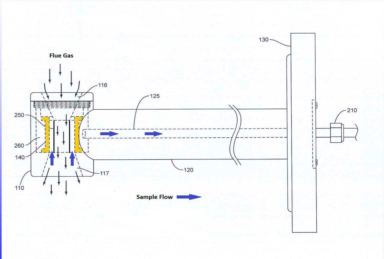
**Separate Sample and Purge Lines, ensures lines and sintered filter are kept clean.**
