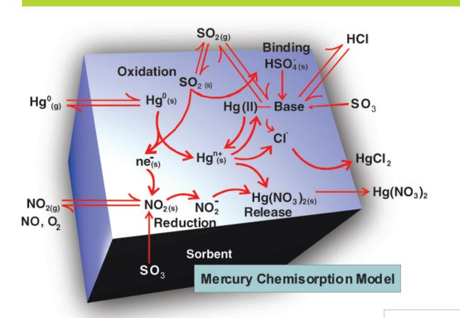
The UND- EERC's chemisorption model for mercury—flue gas interactions with sorbents is both descriptive and predictive.
