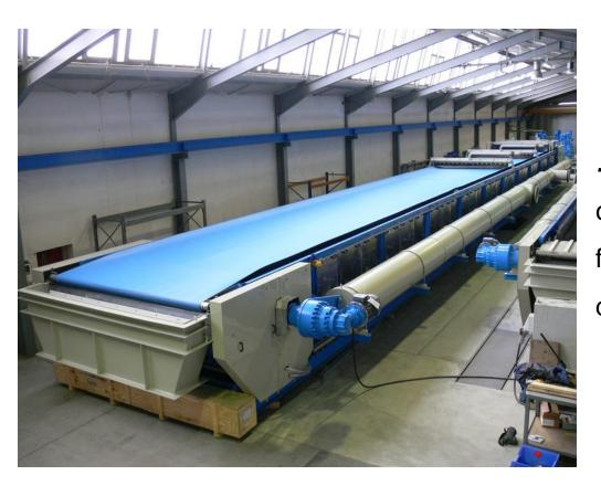
... followed by a vacuum conveyor belt filter for the final gypsum flushing and dewatering.
