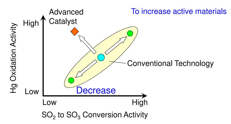
We have developed a new SCR catalyst with Higher Mercury (Hg) Oxidation while maintaining Low SO<sub>2</sub> Conversion
