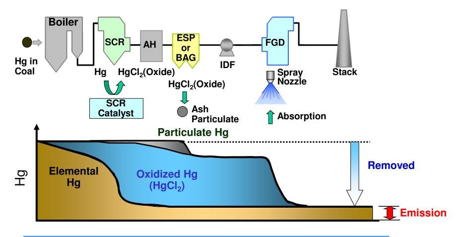
SCR Catalyst is a key component for mercury oxidation
