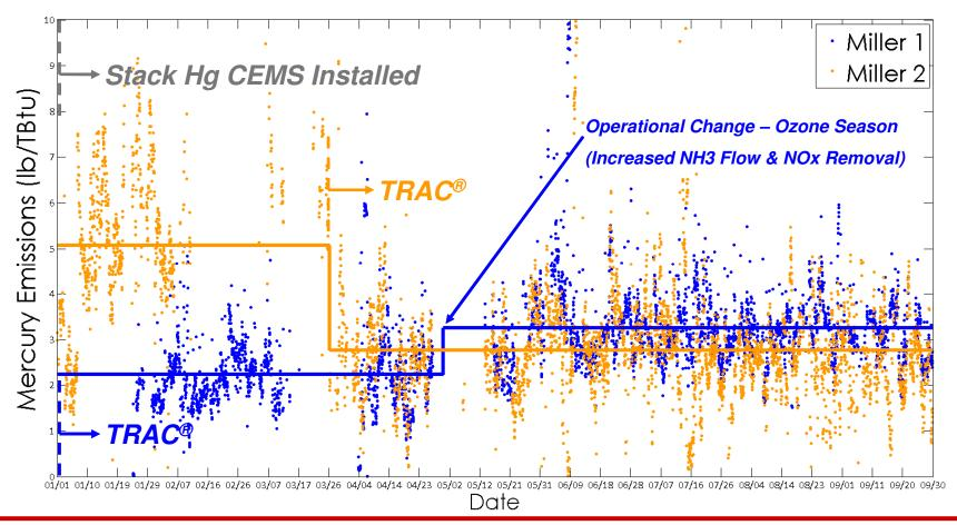
Miller Unit 2 mercury emissions dropped from 5.1 lb/Tbtu to 2.8 lb/Tbtu after installing one layer of TRAC. Miller Unit 1 mercury emissions were 3.3 lb/Tbtu after installing one layer of TRAC.
