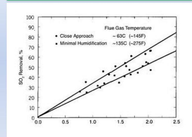
DOE Boiler Trials Using 325 Mesh Limestone Powder
