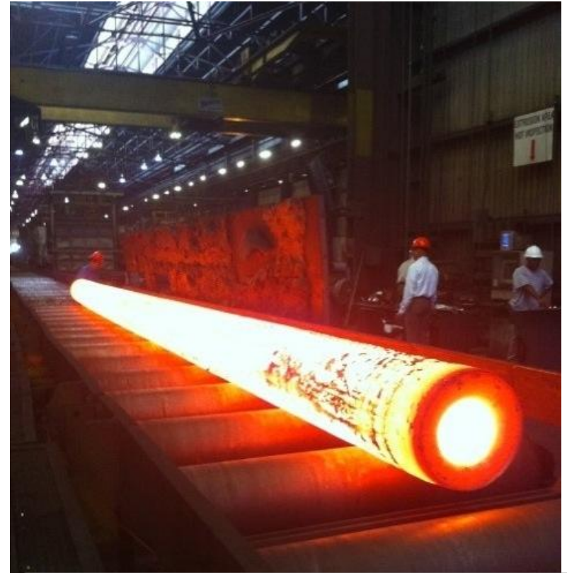
Inconel®740 Pipe after Extrusion at Wyman-Gordon
