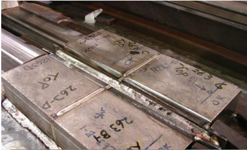
Cast Plate During Welding
