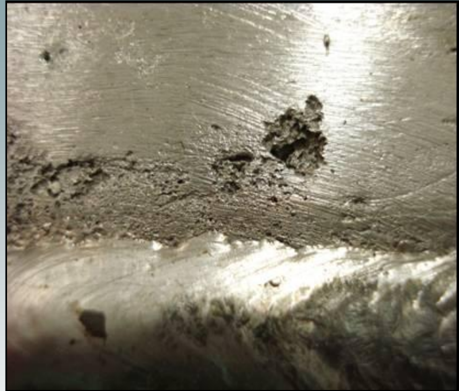
Duplex steel test panel after cleaning. Attack is evident, especially near the weld.
