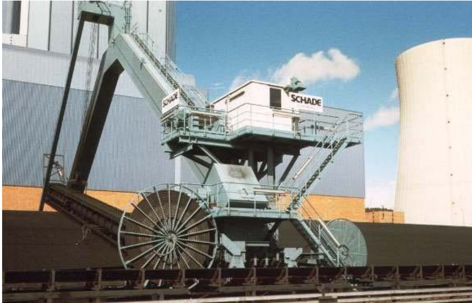
Portal Reclaimer (discharge via drag trough)
