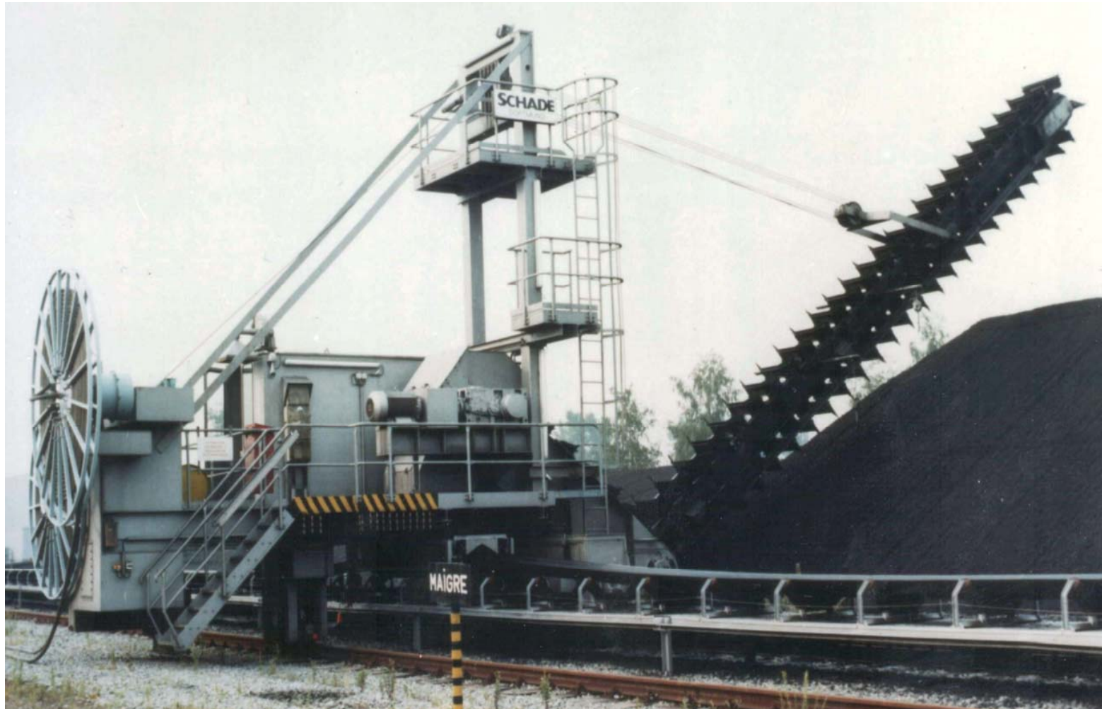
Cantilever Reclaimer (discharge via drag trough)
