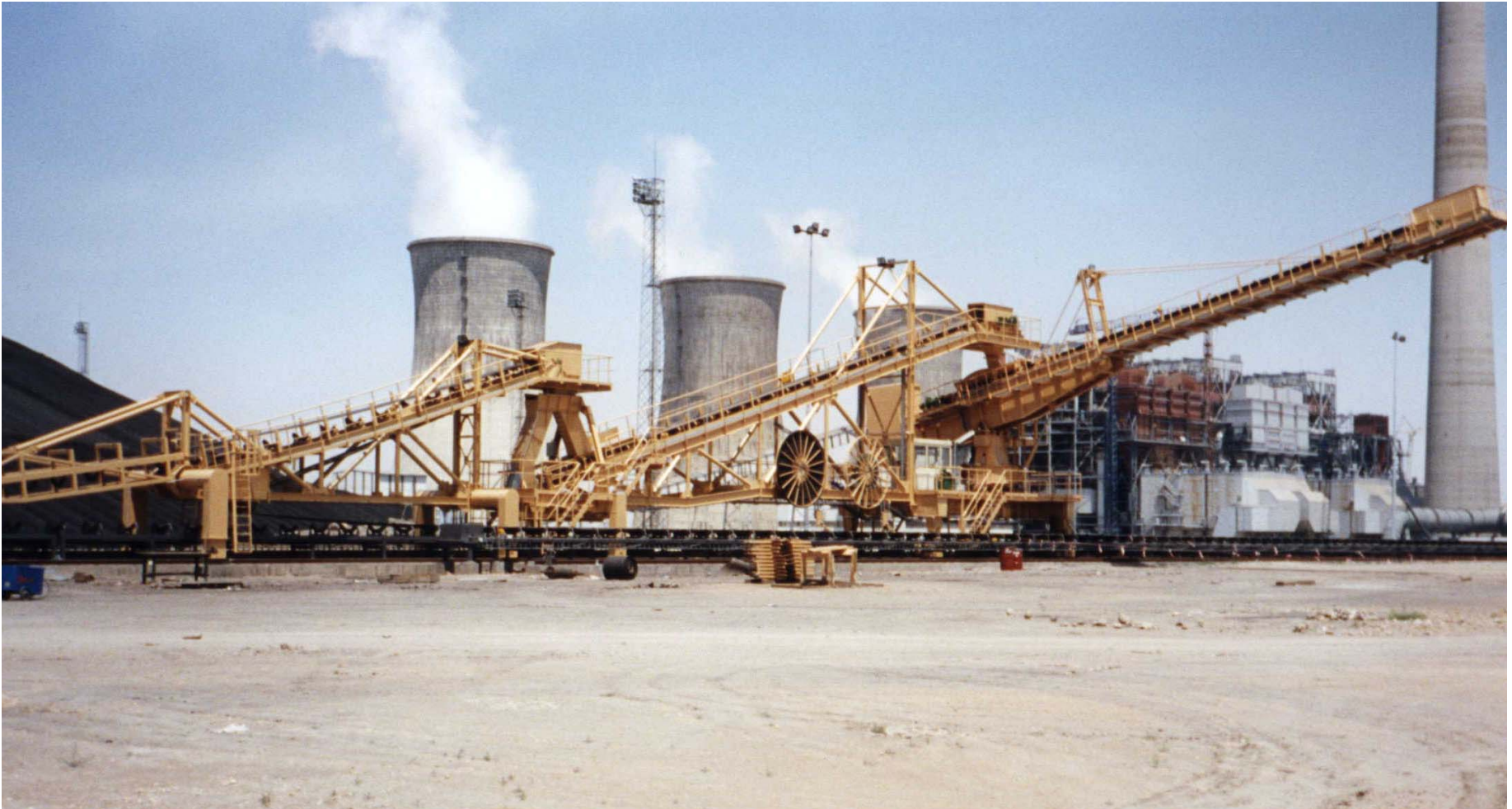
Stacker, slewing and luffing (hydraulic) with by-pass unit
