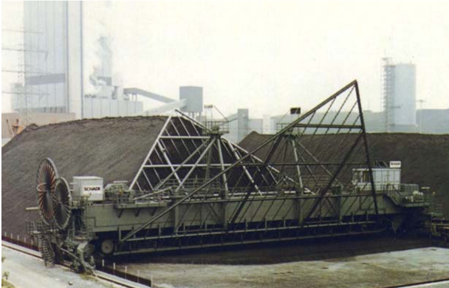
Bridge Reclaimer (discharge via drag trough)
