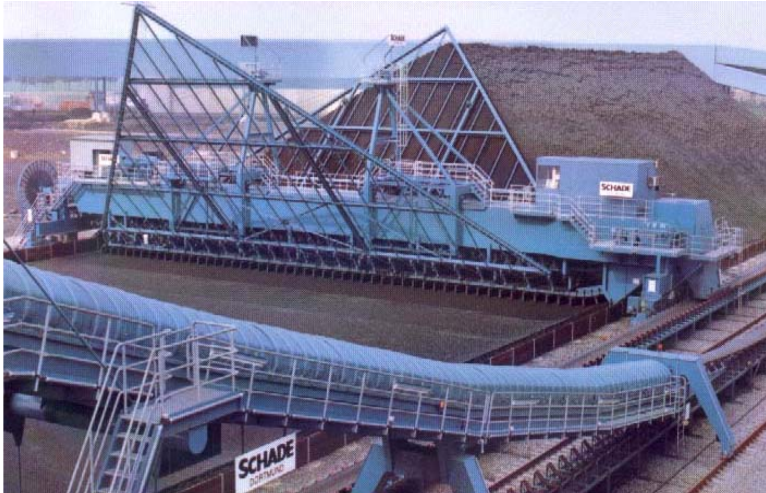
Bridge Reclaimer (discharge via drag trough)
