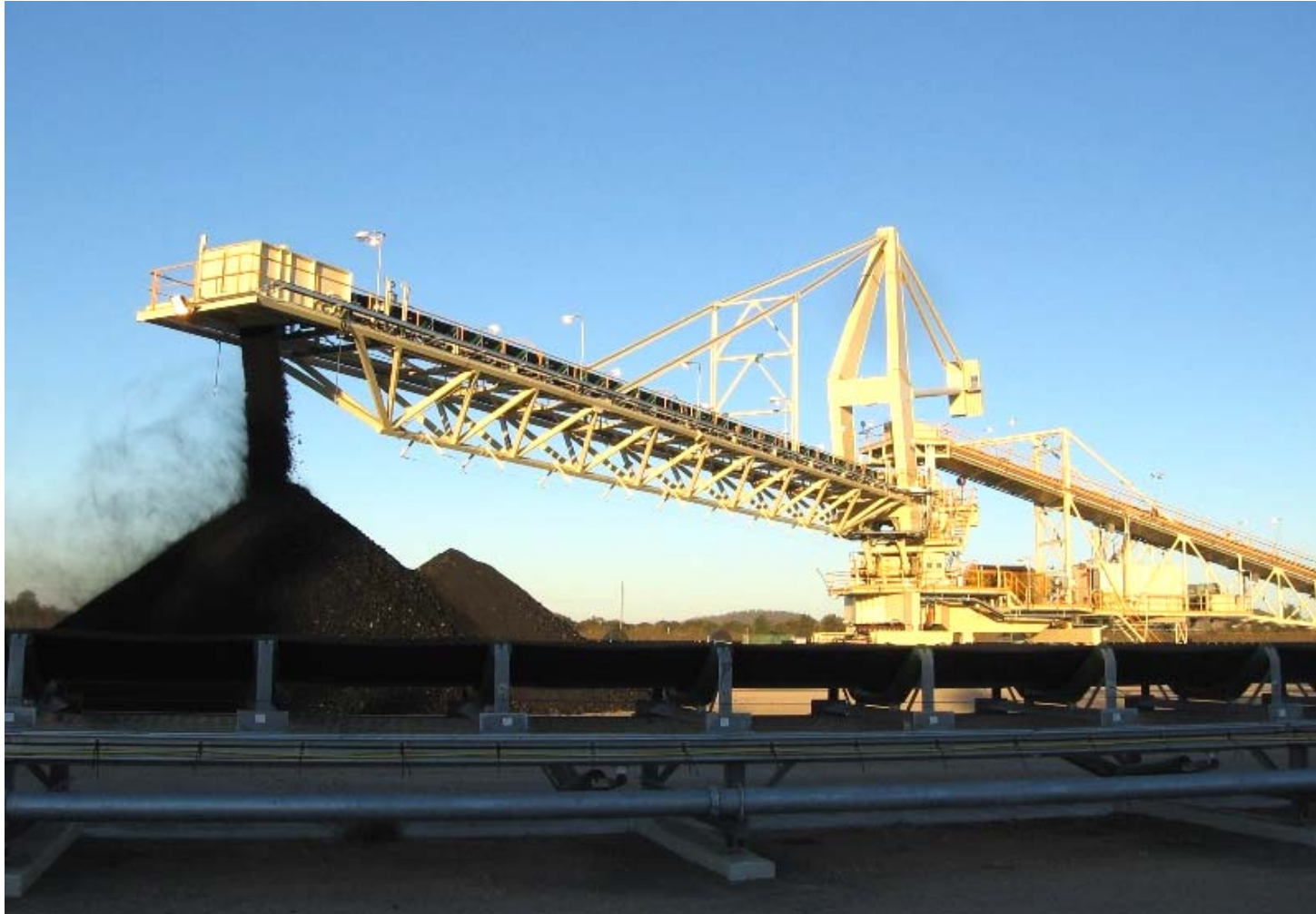
Stacker pylon type, slewing and luffing (hydraulic)
