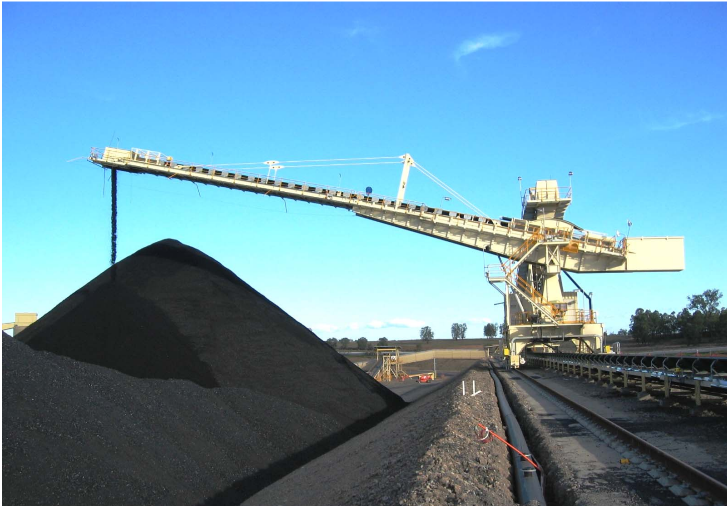
Stacker, slewing and luffing (hydraulic)
