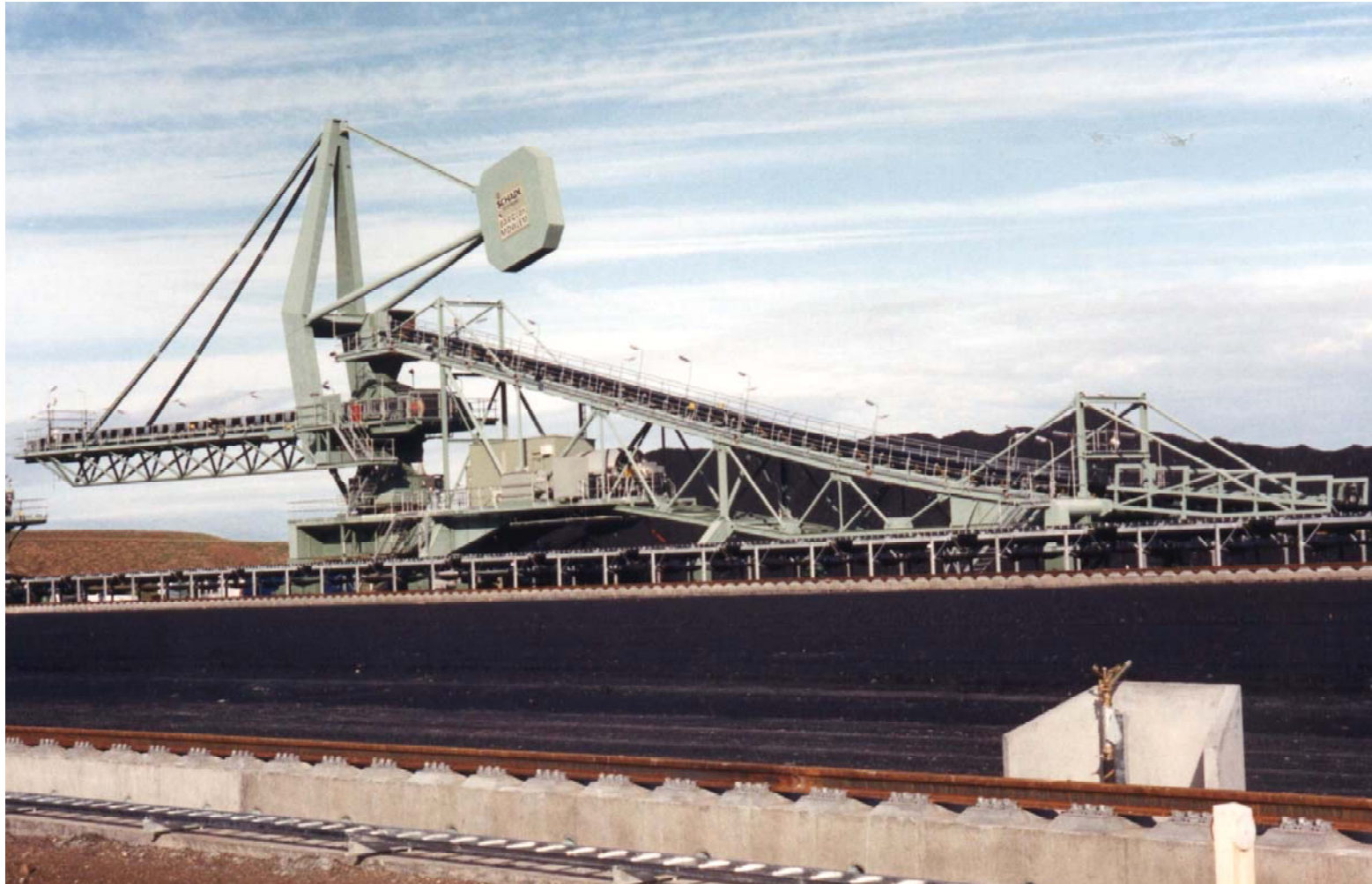
Stacker pylon type, slewing and luffing (hydraulic)
