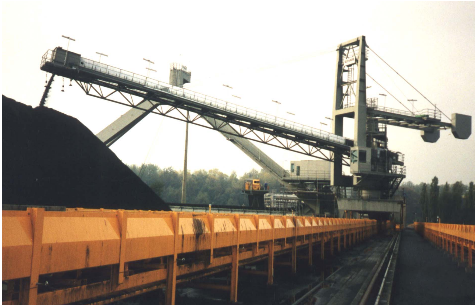
Stacker pylon type, slewing and luffing (rope hoist)
