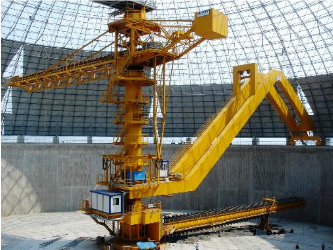
Stacker (slewing) with Semi-Portal Reclaimer (slewing and luffing)
