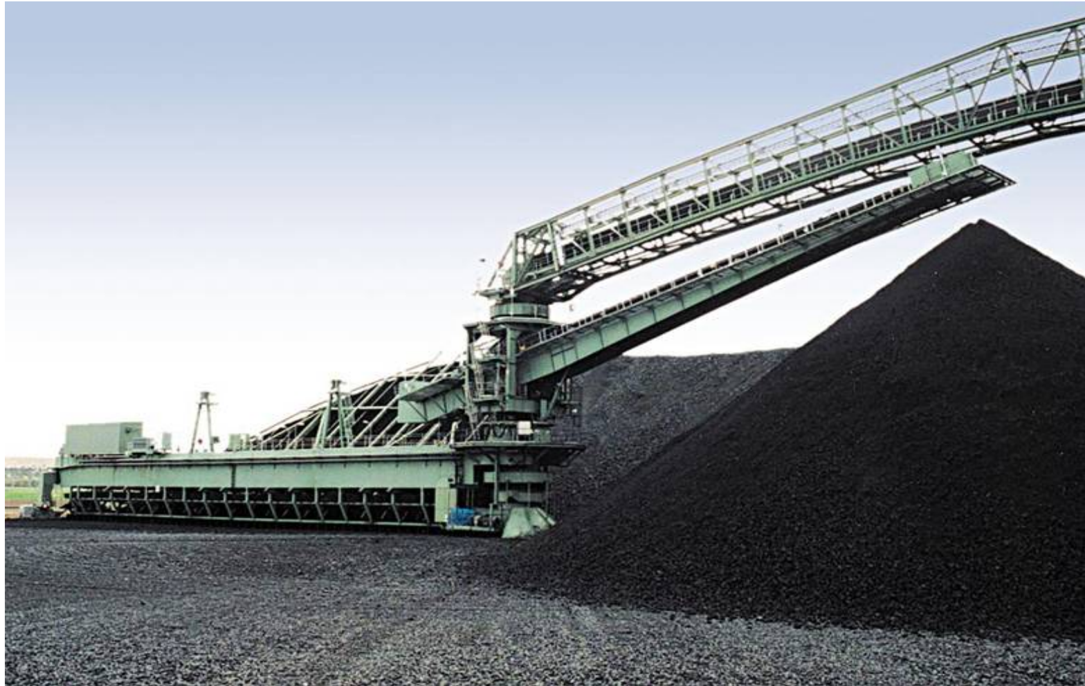
High Capacity Circular Blending Bed dia. 120m
