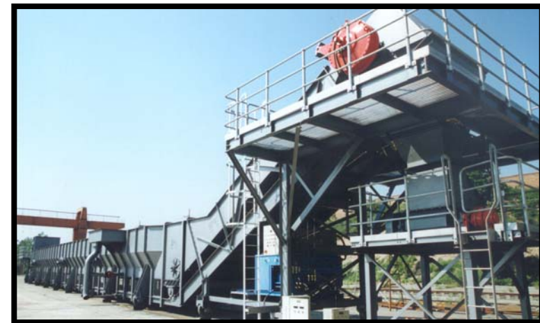
SUBMERGED SCRAPER CONVEYOR
