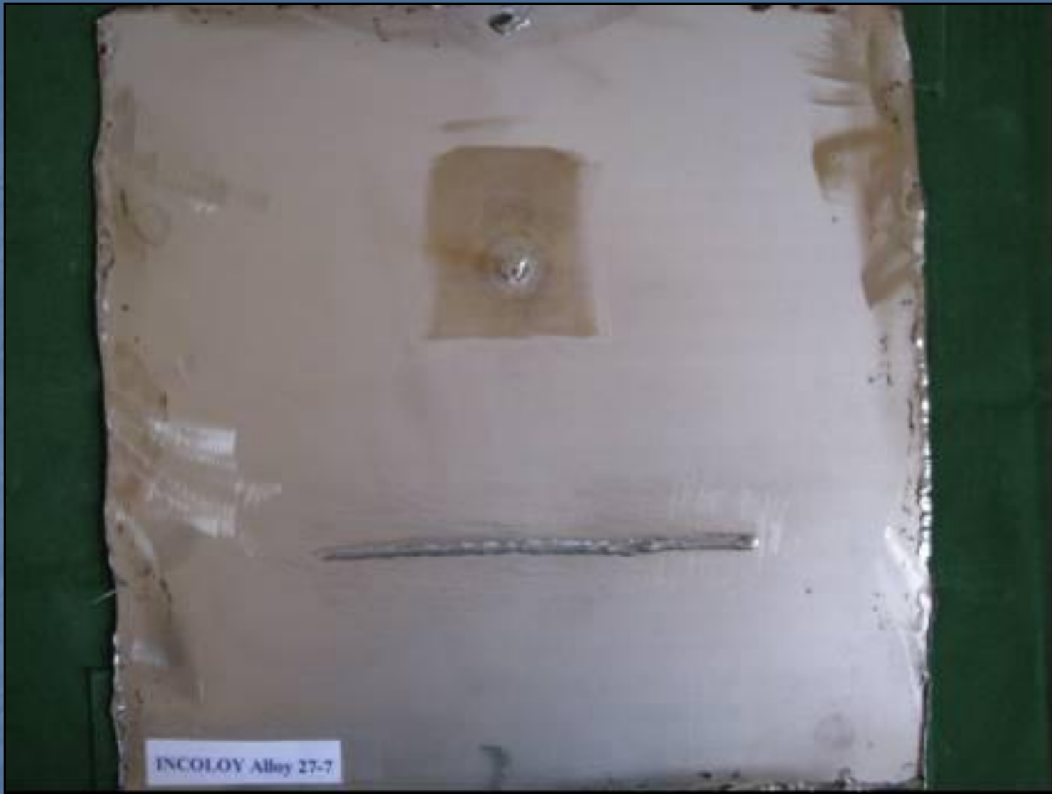
Super-austenitic steel (Alloy 27-7Mo) test panel after cleaning. No attack was found.
