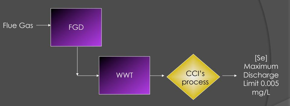
CCI's proprietary process can be integrated following conventional waste water treatment to remove Se.
