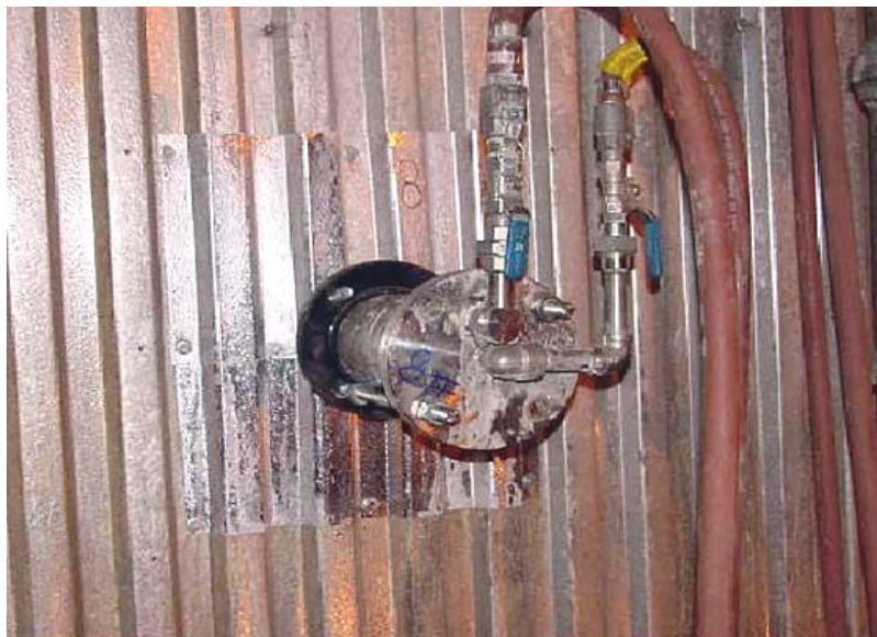
Injector with air supply
