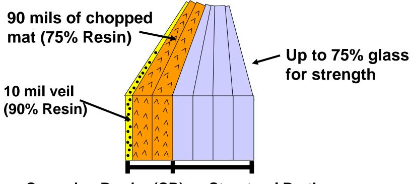
Corrosion Barrier (CB) Structural Portion 100 mils minimum required
