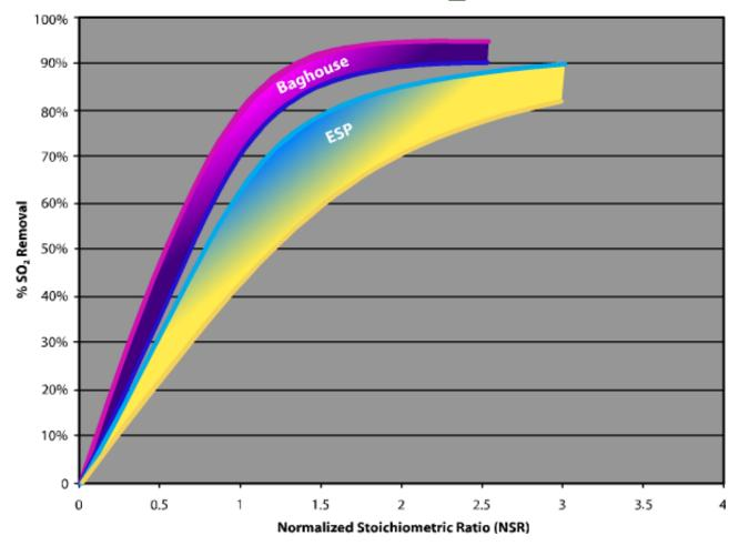
@ 80% SO2 Removal HCl Removal is 98% With NSR of 1.0
