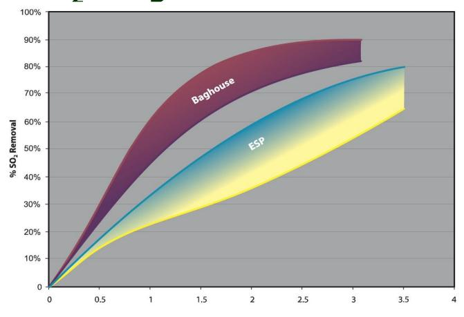
@ 80% SO2 Removal HCl Removal is 98% With NSR of 1.0
