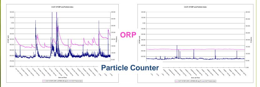
ORP measurements made with the NCSM correlate tightly with measurements made with a particle counter.
