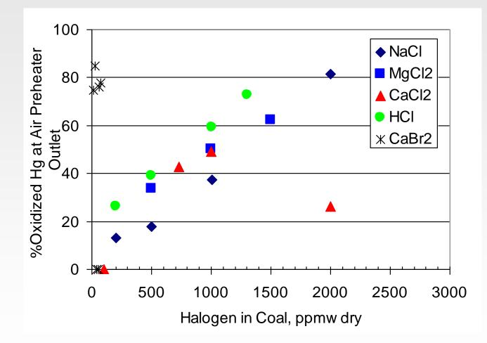
Halogen addition at various full-scale PRB boilers
