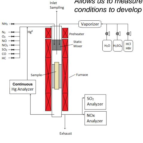
Allows us to measure Hg oxidation under a full range of conditions to develop catalysts and management strategies.
