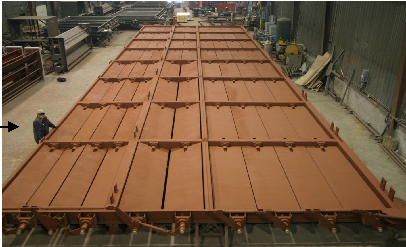
Boiler exhaust -- SH and RH control damper LAVAL SHOP
