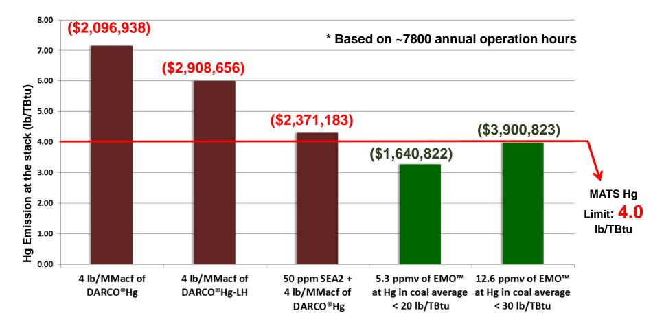
The cost estimates for the first 3 non-EMO<sup>™</sup> injection options were based on Hg Content in coal ~20 lb/TBtu. None of them demonstrated MATS compliance!
