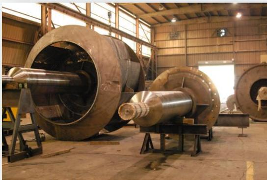
Do ultrasonic testing on all shafts and hubs.
