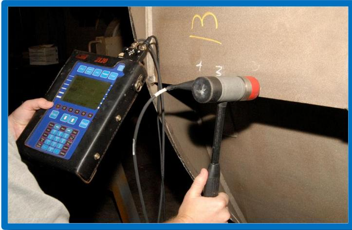
Perform a natural frequency evaluation to prevent a resonance in the rotor with known forcing function (operating speed, blade pass, harmonics, etc.)
