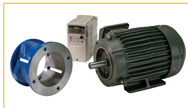
Figure 2. Typically less expensive than electronic actuators, variable frequency drive (VFD) motors and controllers provide full stroke length, thus improving accuracy, eliminating lost motion, and eliminating a potential leak path in metering and dosing applications.
