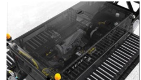
The fully enclosed powerunit offers maximum protection while allowing easy access for daily maintenance
