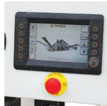
Local machine control panel
