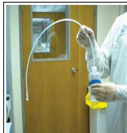
Figure 1. High-purity water PFA Sampler. The sampler uses no O-rings or moving parts allowing for ultra-clean sample collection.
