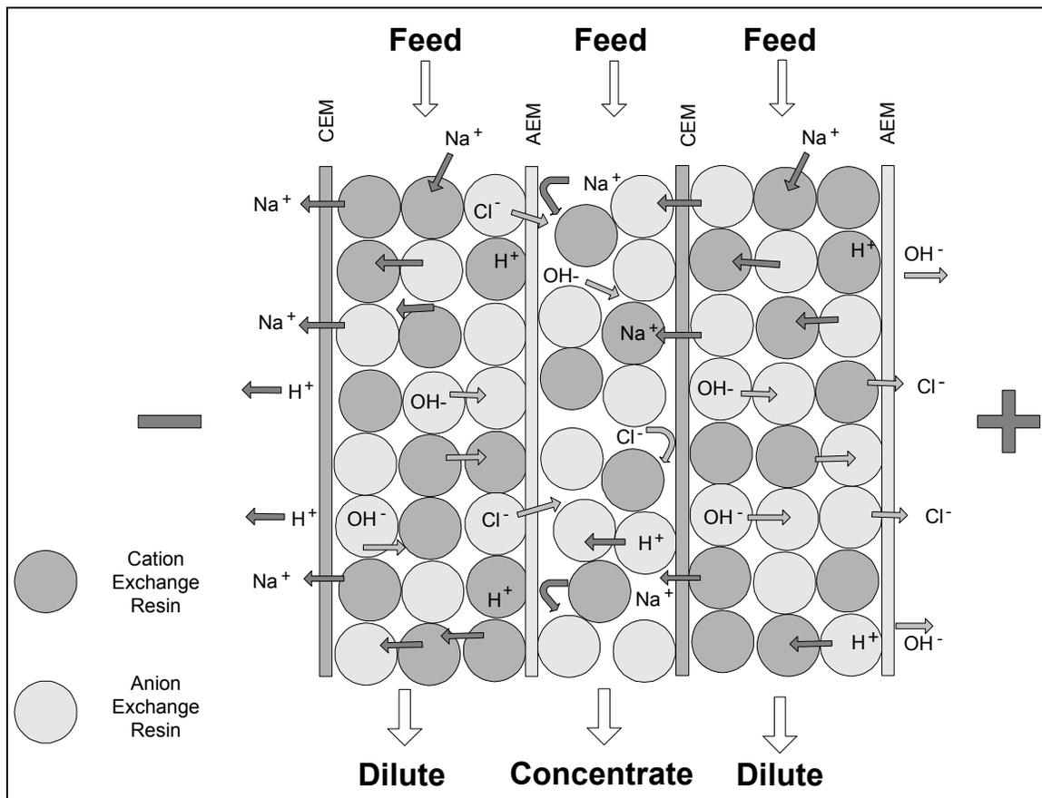
**Figure 2. Water Splitting in Layered CEDI**
