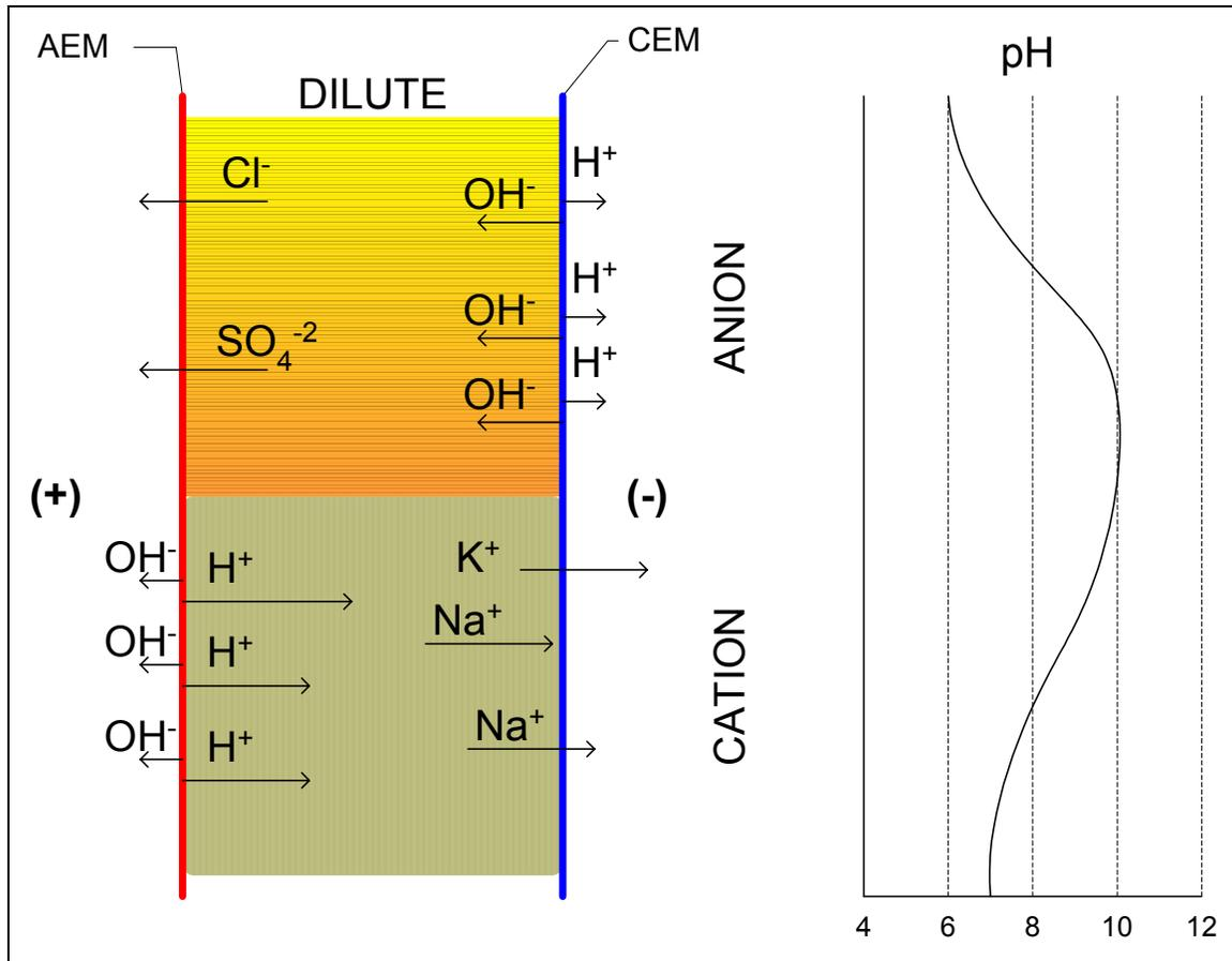
**Figure 3. Theoretical Maximum Bulk pH Increase in an Enhanced Anion Layer**
