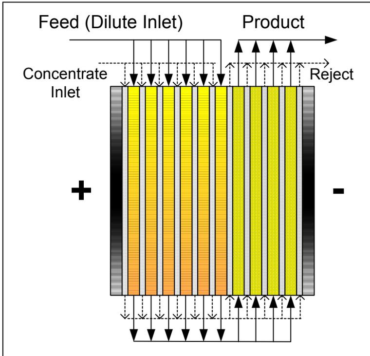
**Figure 5. Two Pass CEDI Using Multiple Modules or Systems**
