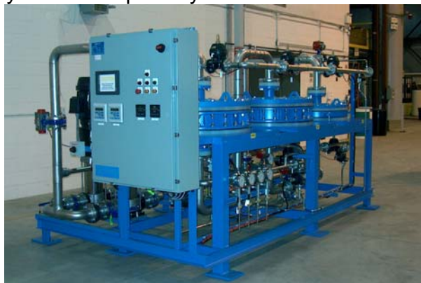
Figure 6 – Single train, skid-mounted, compressed bed system.
