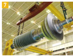
7 M501J Gas Turbine
