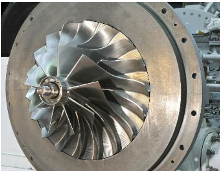
IMPELLER: Induced backward curved vane impeller.
