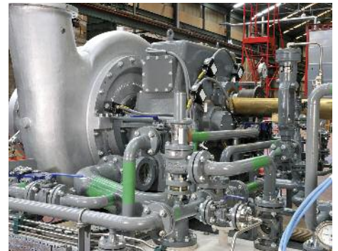
INSTRUMENTATION: Optional API Lubrication System.
