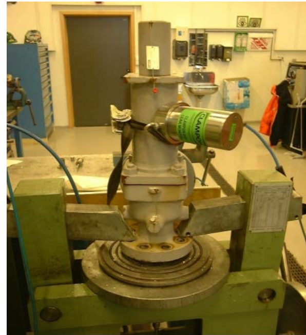
Picture 1, A Leak Monitor mounted on a PSV in the pressure bench at Statoils Kollsnes Refinery.
