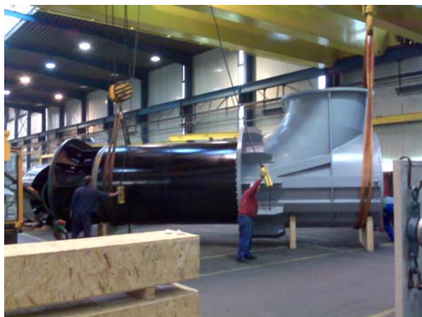
Figure 1. The RKZA pump during assembly
