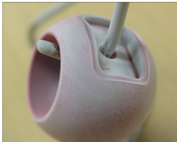
Fig. 8 Coating #1, #2, and #3 were repeatedly subjected to thermal shocks going from ambient temperatures to 675 °C. Then they were put through liquid penetrant tests to check for any cracking
