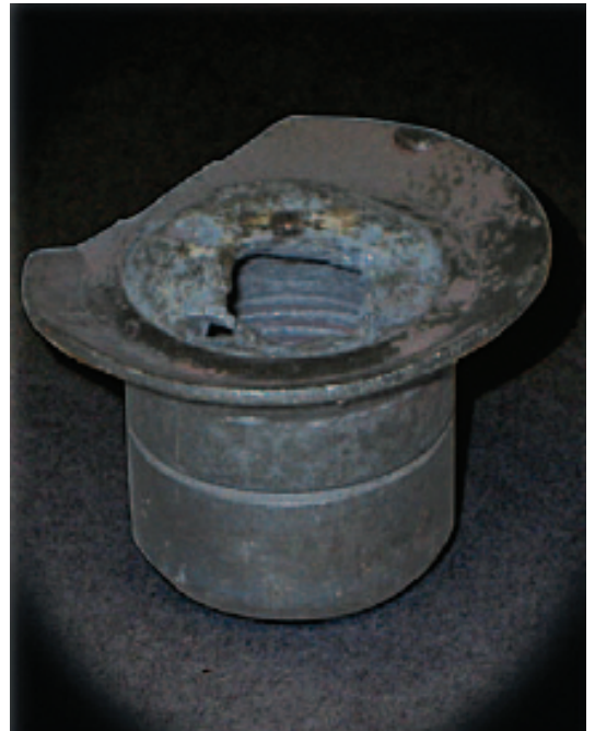
A fouled burner tip
