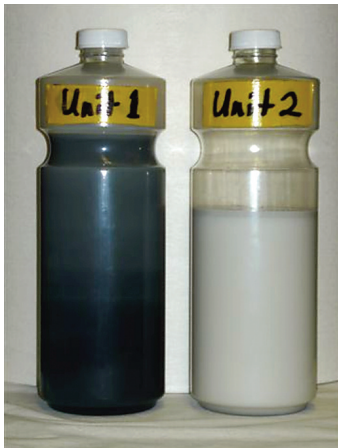
Figure 12. Used Washing Effluents. Unit #1 with 1,450 Firing Hours with F9 Filters Installed. Unit #2 with 2,500 Firing Hours with HEPA Membrane Composite Filters Installed.
