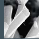
SEM of well developed hexagonal crystals of cement hydration products (x 10,000) Photo: Cementech
