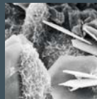
SEM of hydration products in cement (x 1,500) Photo: Cementech
