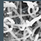
Scanning Electron Micrograph (SEM) of fibrous calcium silicate hydrate products in cement (x 5,000) Photo: Cementech
