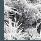
SEM of radiating clusters of cement hydration products (x 1,000) Photo: Cementech
