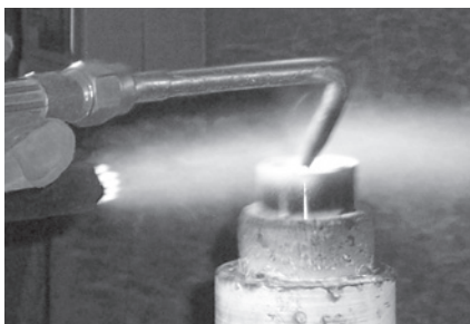
Using the latest technology, this seat is receiving a coating. MOGAS coatings are specially chosen to handle the operating conditions of each application.
