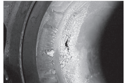
As shown in this competitor's valve, if seats are not protected from constant exposure to high pressure steam, destructive erosion can occur.
