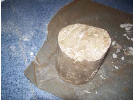
FIGURE 3. Ottawa River sediment waste treated with class C fly ash/type I/II Portland cement to form a monolithic material.
