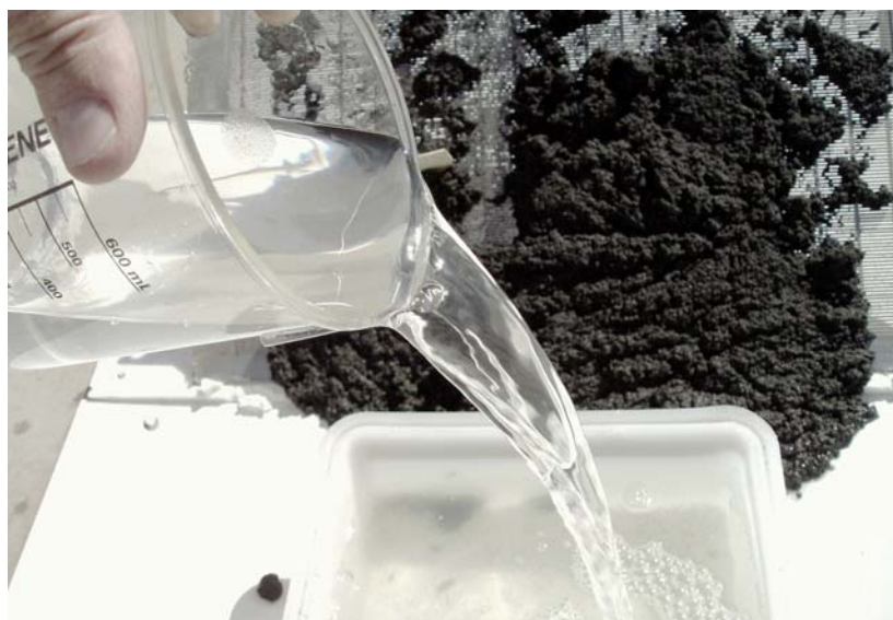
FIGURE 2. Dewatered sediment from Ottawa River and filtrate collected under the screen (at 15 NTU with “trace” suspended solids).
