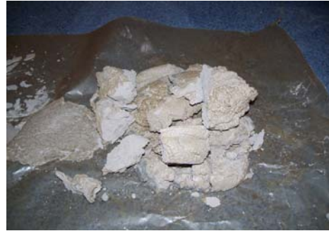
FIGURE 4. Ottawa River sediment waste treated to create an aggregate material.
