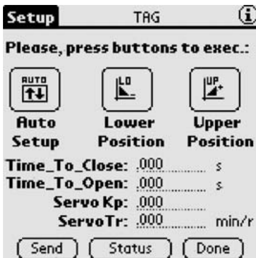
FIG. 6.11g The display of a handheld tool for configuring a digital valve positioner. (Courtesy of SMAR; the screenshot is of SMAR HPC301.)
