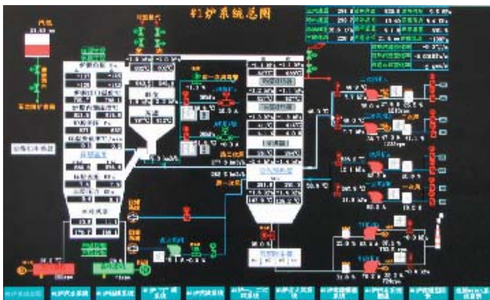
SIS boiler operation display
