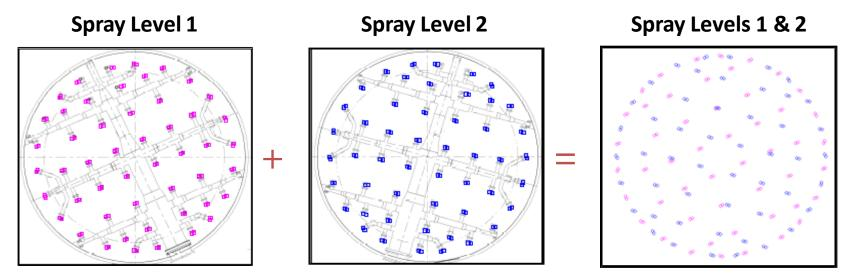
Adjacent levels are offset from one another to provide complete coverage, prevent channeling, and minimize wall sneakage.
