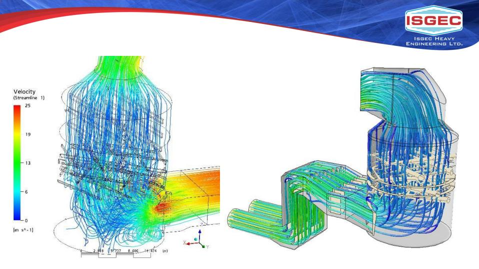
Inlet duct design and spray pattern, spray nozzle placement and wall ring prevents channeling and distributes gas over the entire cross section while delivering even slurry spray.
