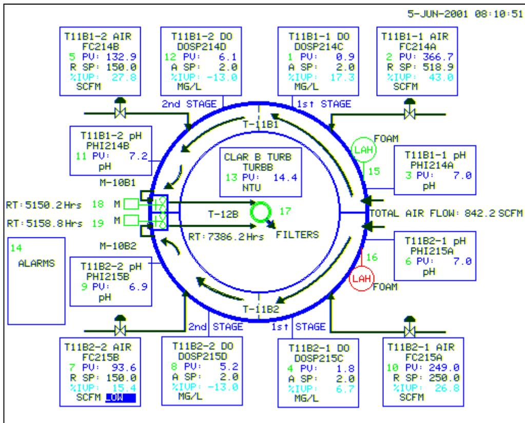
**Figure 2 Computer Display of Aeration Tank Instrumentation and Controls**
