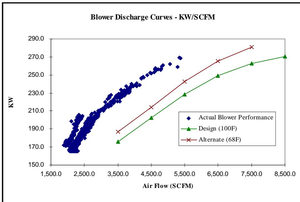
**Figure 6 300 HP Centrifugal Blower Curves, Actual and Two Design Conditions (68F and 100F)**
