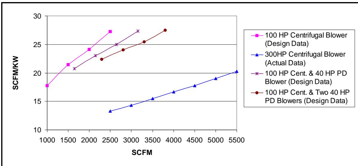
**Figure 8 Operational Scenarios possible with One 100 HP Centrifugal Blower, Two 40 HP PD Blowers, and One 300 HP Centrifugal Blower**
