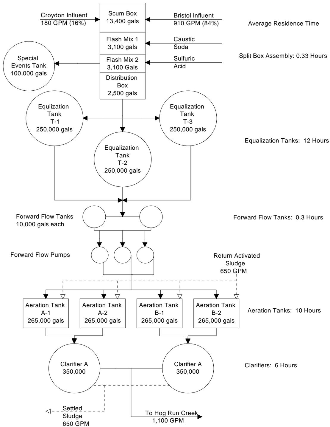
**Figure 1 Flow Diagram for Rohm and Haas Bristol/Croydon Complex WWTP**
