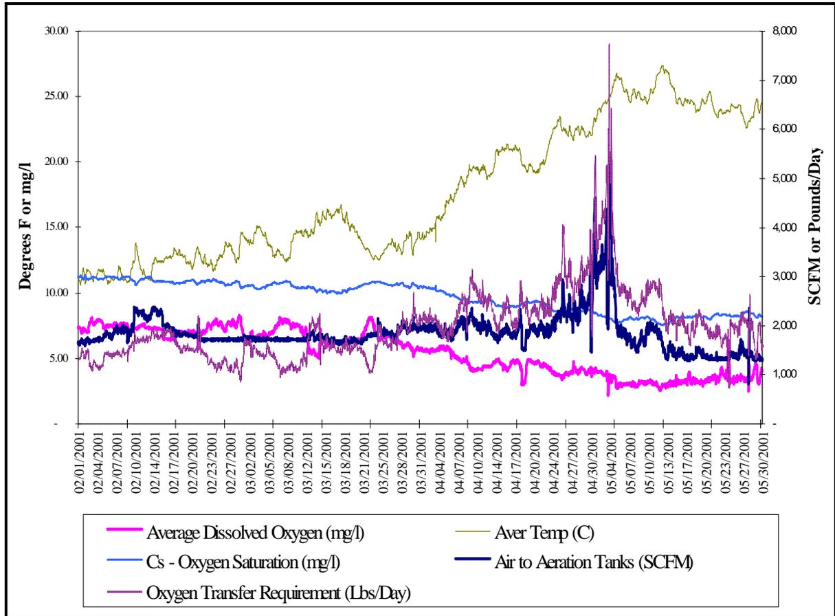
**Figure 4 Hourly Average Data on Aeration System Performance collected between May and June 2001**
