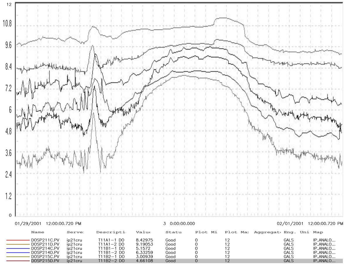
**Figure 9: Dissolved Oxygen (mg/l) versus Time demonstrating Inhibitory Substance elevating Dissolved Oxygen Levels (Screen Print from Data Acquisition System)**
