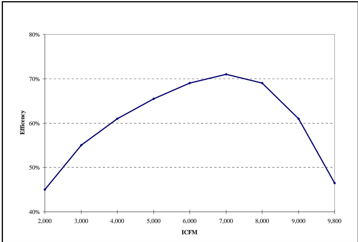
**Figure 3 Graph of Mechanical Efficiency of 300 HP Blower**
