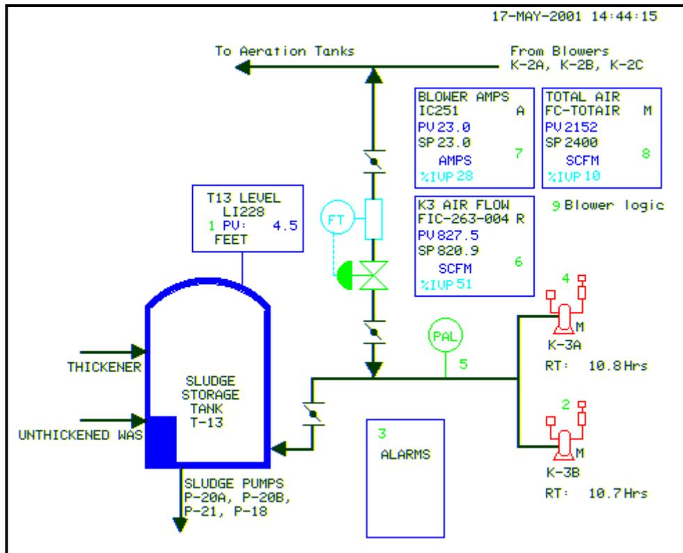
**Figure 7 Computer Display of Sludge Holding Tank with new Connection to Main Aeration Blowers and Current Controls**
