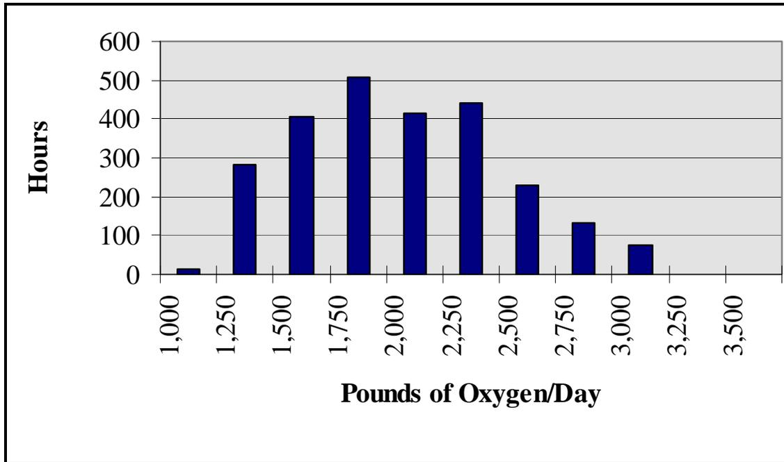
**Figure 5 Pareto Analysis of Hourly Average Oxygen Transfer Data collected between May and June 2001**
