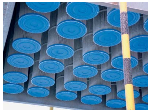
TFP95 cartridges functioning under icy conditions
