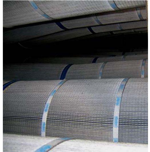
Viledon cartridges GTC 327+445 after 1000 h
