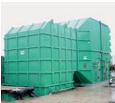
Large filter house module
