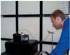
Measuring the clean-gas-side volume flow and the raw-gas-side particles
