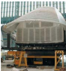
An assembled intake air filter housing, with an up-stream water separator
