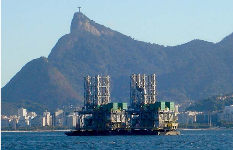
4 of 12 air intake systems (278,000 m 3 /h each) on their way to assembly on an offshore platform (Brazil)
