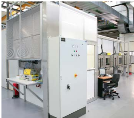
Filter test channel to EN 779 in Freudenberg's metrological laboratory
