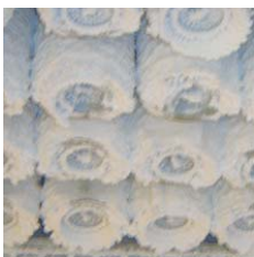
Blocking, non-pulsable ice layers on the competitor's cartridges previously used at -15 to -20^{\circ}\text{C}
