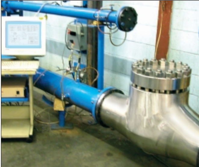
Flow testing on a 10" Class 1500 forged bolted cover swing check valve.
