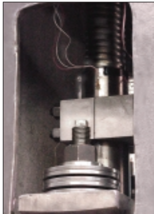
Velan delivers valves with preinstalled thrust and torque sensors, signal conditioners and cabling (smart stems).
