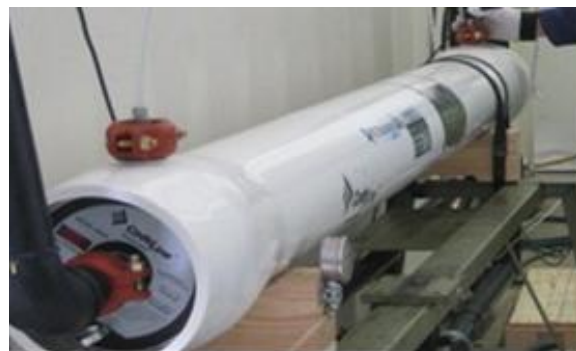
8x80-inch Liqui-Cel® Membrane Contactor at the RO Solutions Test & Pilot Facility in Norway
