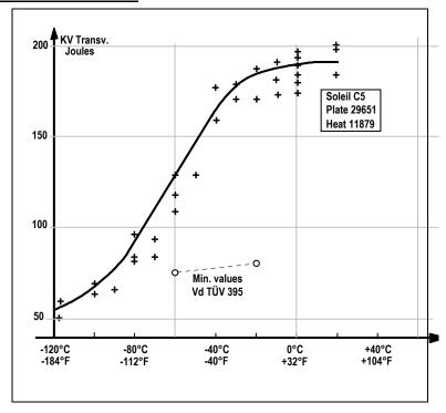
Soleil C5 alloy presents improved toughness properties when compared to ferritic-martensitif grades (AISI 410-420/ EN 1.4000-X6 Cr 13).
