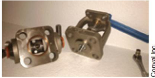
1. Manual ball valve has removable top for maintenance and inspection. The copper-coated ring is the body-to-bonnet seal
