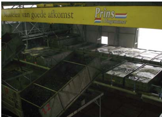
▲ The unloading platform where containers from the ships are placed above the flush platform
